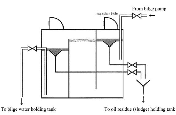
Figure 1 – Example of a bilge primary tank
