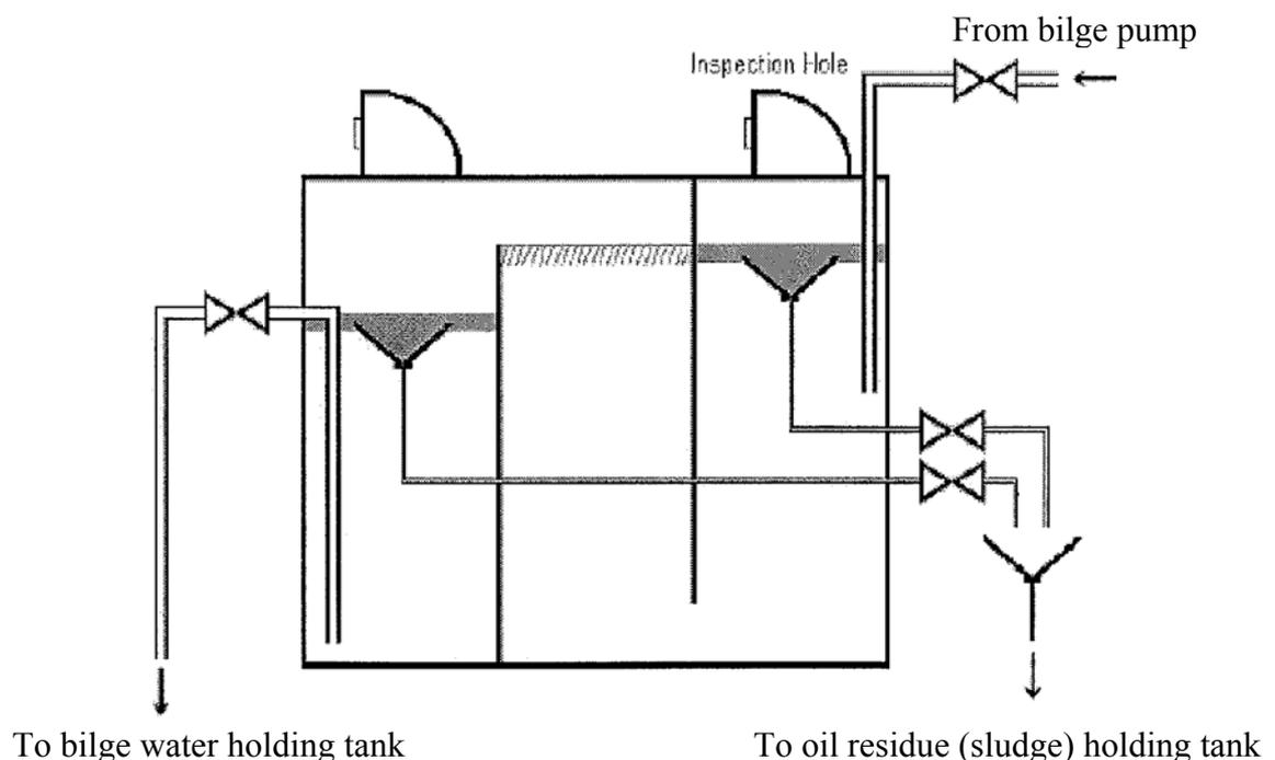
**Figure 1 – Example of a bilge primary tank**
